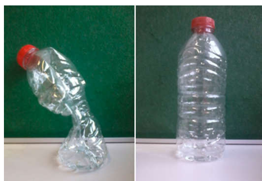
Figure 5. Plastic bottles filled with sodium hydroxide solution and CO 2 (left), and filled with sodium hydroxide solution and air (right). The NaOH solution absorbs CO 2 but not air, hence only the bottle that contains CO 2 has contracted. This interactive demonstration helped support the explanation that liquid solvents could absorb gaseous CO 2 .
